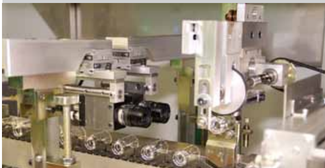
In process camera-controls
